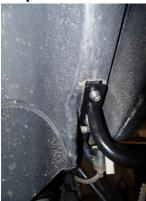
Attach the right hand bracket under the seat, (Bracket is longer to pass under the petrol tank.)
