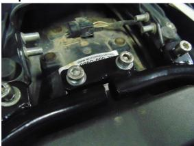
Fix the two pannier frames together with the supplied bolts and nutx.
