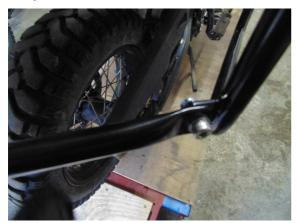
Attach the rear brace between the two racks with the supplied bolts and nuts.
