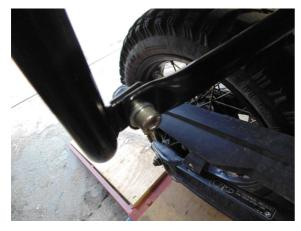
Attach the pannier frame to the previously installed bracket using the supplied Bolt and nut.
