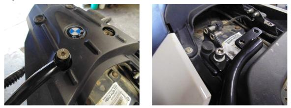
Attach the Right hand Pannier frame using the countersunk bolt on the rear bracket. Use the bolt taken from the BMW rear rack on the front hole.
