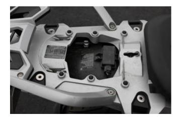
3. Place the 4 brackets in the areas as shown and return 4 bolts which you removed in step 1.
