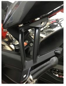
5. Attach the exhaust back. Provide clearance between the bolt and swing-arm as shown on the picture :
