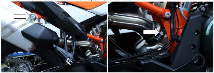
3. Remove the three bolts shown on the picture together with the passenger foot peg both sides.
