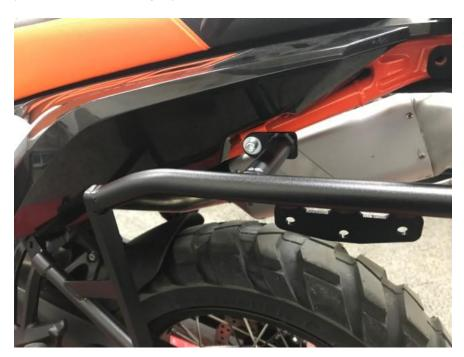
7. Attach the pannier rack using M8 x 60 mm , washer M8 and Aluminum spacer  $\phi$ 15 x 20mm as shown on the picture. Do not tight them yet.
