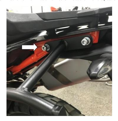
9. Attach the front point of the frame to the passenger foot peg bracket using M8 x 20 mm, 2 x washer M8 and and M8 Self- Locking nut. Do not tight yet.
