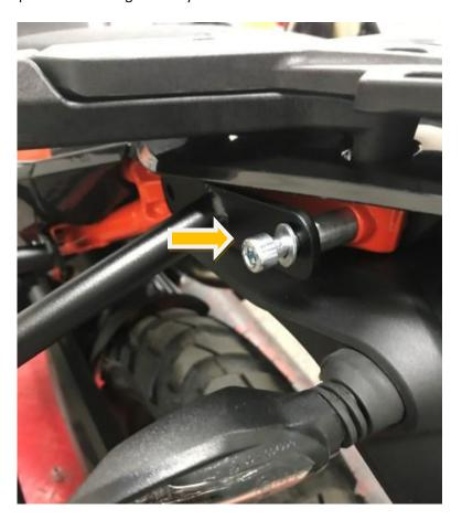
8. Mount M8 x 20mm bolt with washer M8 as shown on the picture
