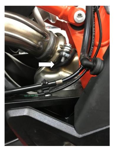
6. Attach the Pannier racks using M6 x 15mm with washers M6 x 18 and M6 Flange Nut as shown on the picture. Please do not tight yet.
