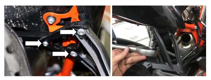
4. Put 2 x aluminum spacers φ20 x 7/ 14mm and bracket as shown on the picture. Attach the passenger foot peg with OEM bolts back. The same steps on the right side.
