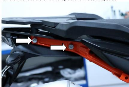
2. Remove the two bolts shown on the picture and the exhaust:
