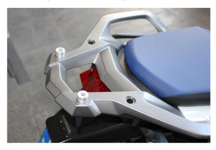
2. Put the top case mounting plate and the four bolts as shown on the picture.
