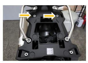
5. Put aluminum spacers  $\phi$ 19 x 9 mm as shown on the picture:
