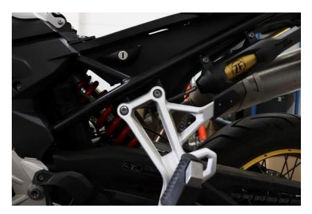
4. Put the aluminum spacers  $\phi$ 19 x 5mm as shown on the picture:
