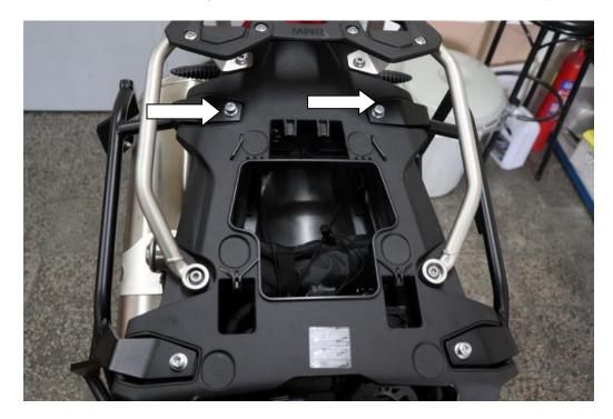
8. Attach the pannier rack to the passenger foot peg using 2 x OEM bolts and Spacer ( powder coated)  $\phi$ 20 x 4mm as shown on the picture:
