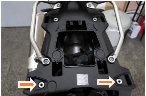
6. Attach the Pannier racks using M8 x 50mm with 2 x washers M8 as shown on the picture:
