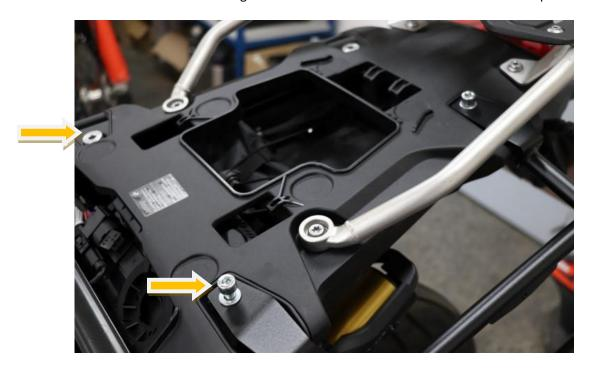
7. Attach the Pannier racks using M8 x 40 mm with 2 x washers M8 as shown on the picture:
